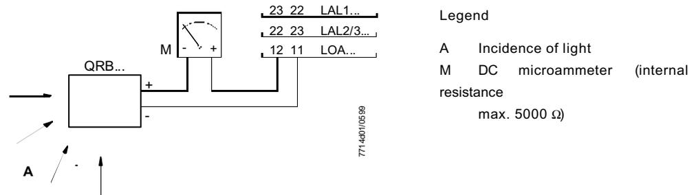
For the minimum detector current values required, refer to the data sheet of the respective burner control.
