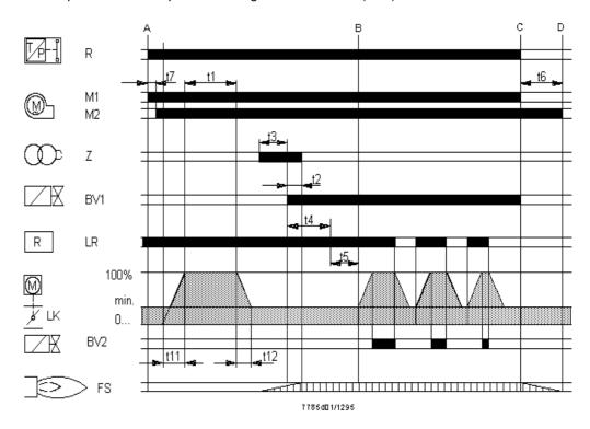
**Interrupted pilot burners** (burners with a pilot burner), controlled and supervised by LGK16.335 or LGK16.635, for example. The other types of burner controls of the LGK16... range program the times «t2», «t3», «t4» and «t9» for the pilot burner.
