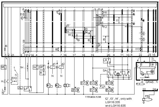
Control signals delivered by the burner control
