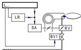
Load control with a modulating controller with galvanically separated control contacts for OPEN and CLOSED positions.
