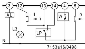
The burner is switched on manually by pressing button «I».
