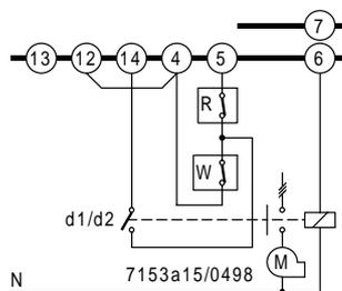
If an auxiliary contact «d1 / d2» of the fan contactor is included in the circuit as shown in the diagram, ignition and release of fuel are possible **only** when the contact is closed.
