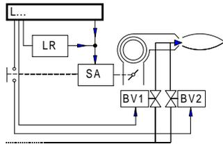
Load control with an on / off controller.
