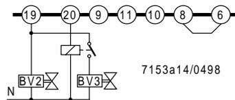
The relay is not required if «BV3» connected to terminal 20 is hydraulically series-connected with «BV2».
