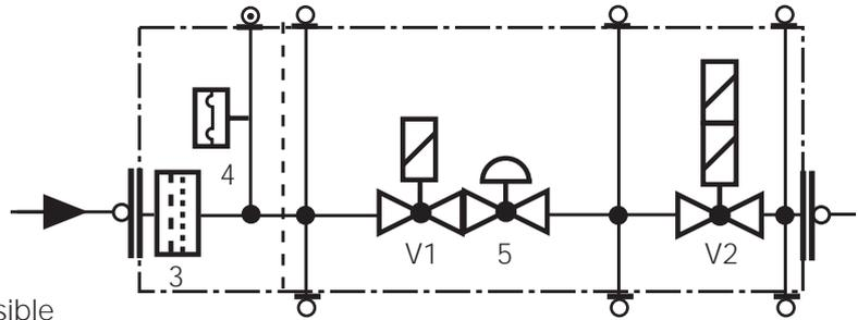
Mounting of VPS 504 valve proving system possible
