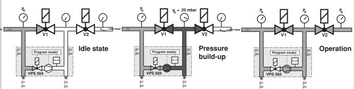
Idle state: Valves 1 and 2 are closed. Pressure build-up: The internal motor pump increases the gas pressure p in the test section by approx. 20 mbar compared to the input-side pressure applied to valve V1.
