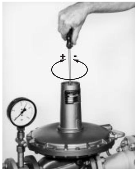
If the SAV close due to a operating fault at the pressure regulator, you can manually open the SAV after eliminating the fault.
