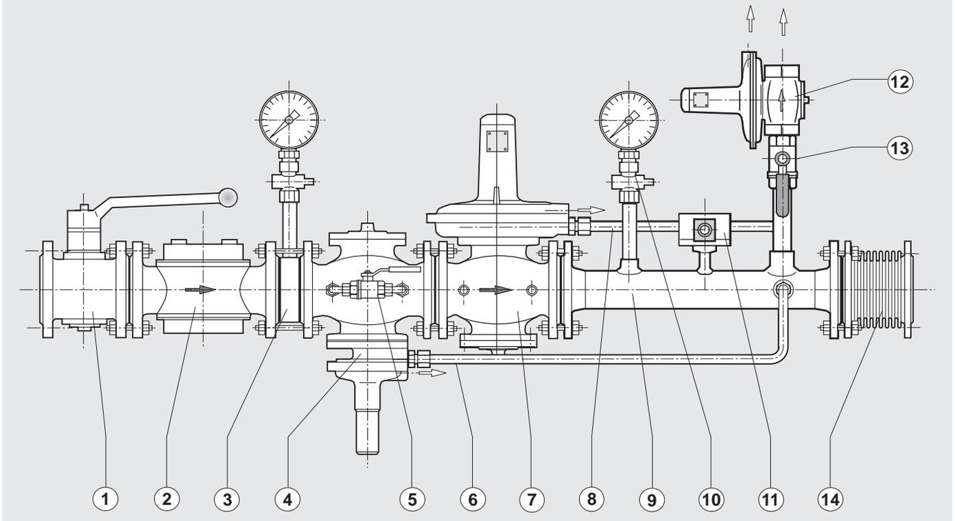
Regulating train comprising RS 250/RS 251 pressure regulator, built-in safety shut-off valve and SL 10 blow-off valve
