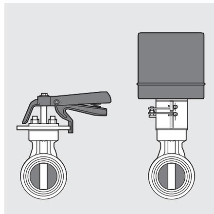
Different setting ranges by means of toothed scale and handle with 90° grid. We supply continuous fine adjustment or motor actuator for the regulating valve. Actuators: Commercial motors can be retrofitted.
