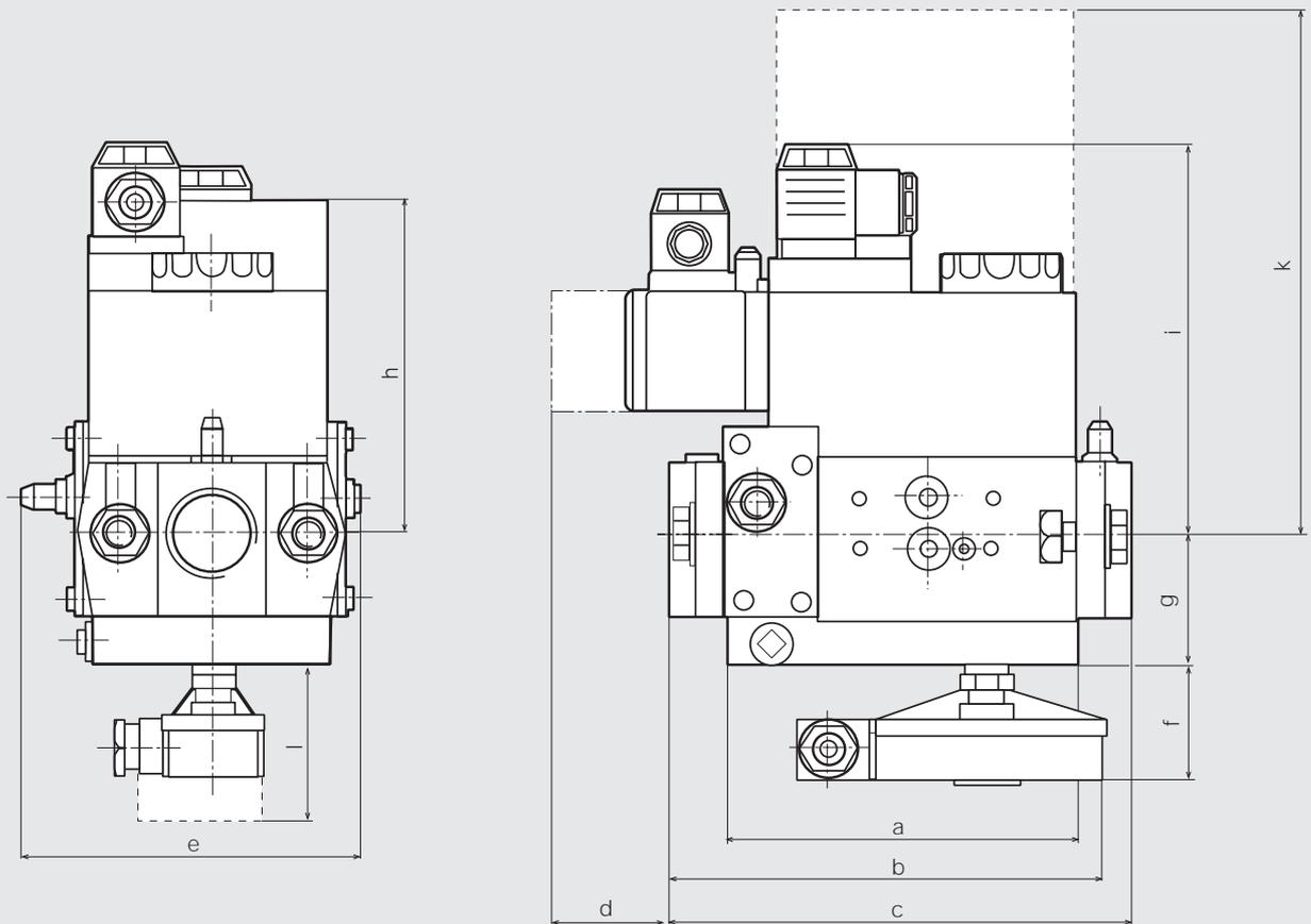
d = Space requirement for cover of pressure switch
