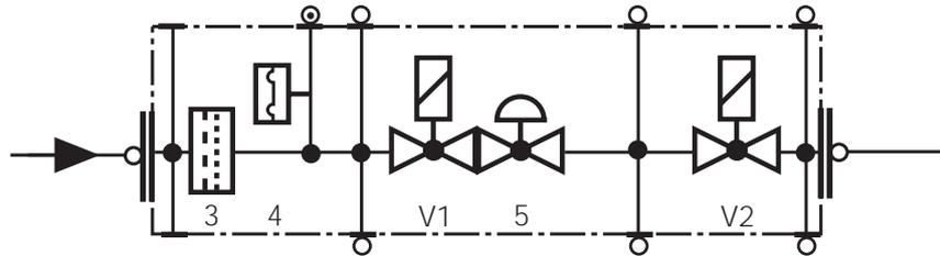
Mounting of VPS 504 valve proving system possible
