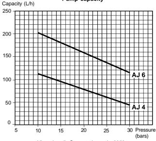
Viscosity = 5 cSt - rated speed = 2850 rpm Data shown take into account a wear margin. Do not oversize the pump when selecting the gear capacity.
