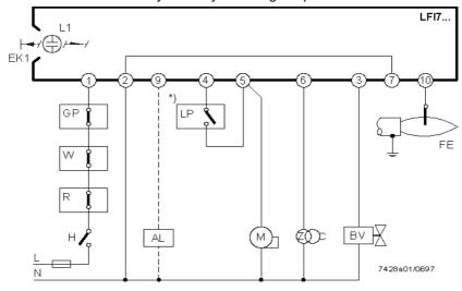
\*) Air pressure supervision not conforming to EN 298!
