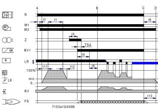
During burner off times, the air damper is closed. When using actuators without changeover limit switch «z» for the CLOSED position, terminals 10 and 11 must be interconnected.
