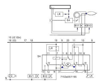
Load control with an on / off controller. During burner off times, the air damper is closed.
