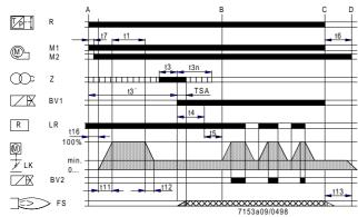
Control of actuator based on single-wire control.
