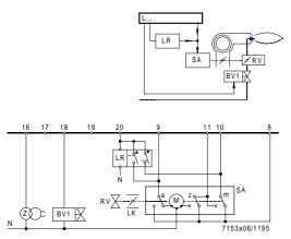
Load control with a modulating controller with galvanically separated control contacts for OPEN and CLOSED positions.
