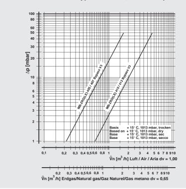
GasMultiBloc Combined regulator and safety shut-off valves Two-stage function Integrated bypass valve
