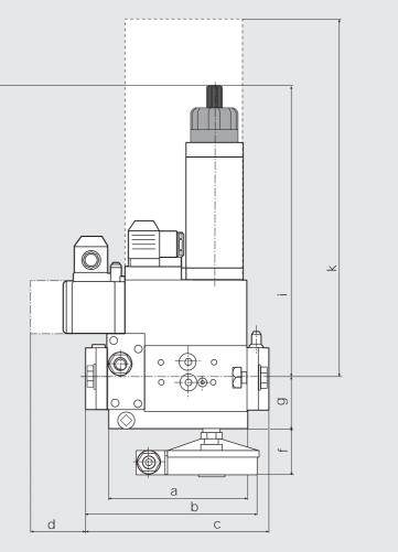
d = Space requirement for cover of pressure switch k = Space requirement for exchanging the solenoid I = Space requirement for K01/1 closed position signal contact
