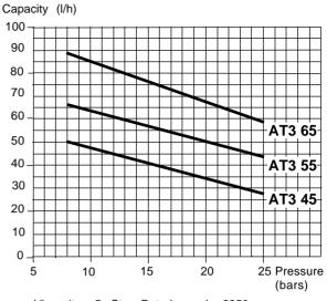
Viscosity = 5 cSt - Rated speed = 2850 rpm
