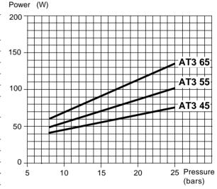
Viscosity = 5 cSt - Rated speed = 2850 rpm
