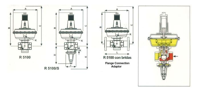
Model R 5100 MP Regulator only and R 5100/S complete with Safety Shut-off Valve.
