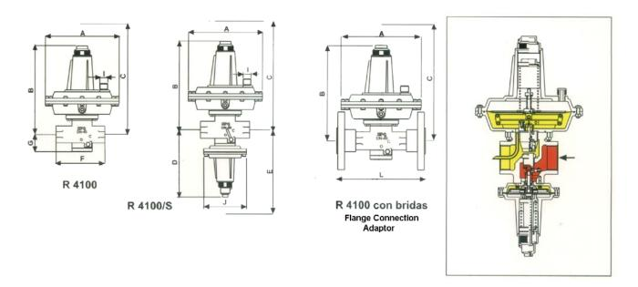
Model R 4100 MP Regulator only and R 4100/S complete with Safety Shut-off Valve.
